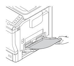
→ If a cap is in the long side of an envelope (western-style envelope #2, western-style envelope #6, or envelope DL), load the cap into the machine side.
