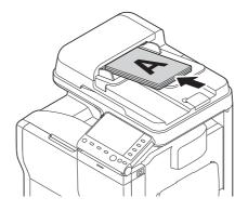
→ Load the original so that its top side is placed at the back. When loading in a different orientation, be sure to specify the loading direction of originals.
