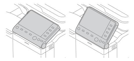
To adjust the angle of the Control Panel, tilt the Control Panel up and down.
